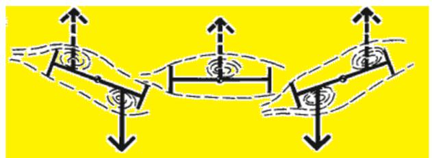
Although the static air loads on the array are always less than its structural strength, once the array begins to twist and bend in a periodic manner, under certain conditions the dynamic air loads may begin feeding the elastic motion of structure, causing its amplitude to grow, which in turn causes increased air loads that eventually exceed the structural strength. Such a catastrophic dynamic coupling between the elastic motion and the unsteady aerodynamic loading is called "flutter".
