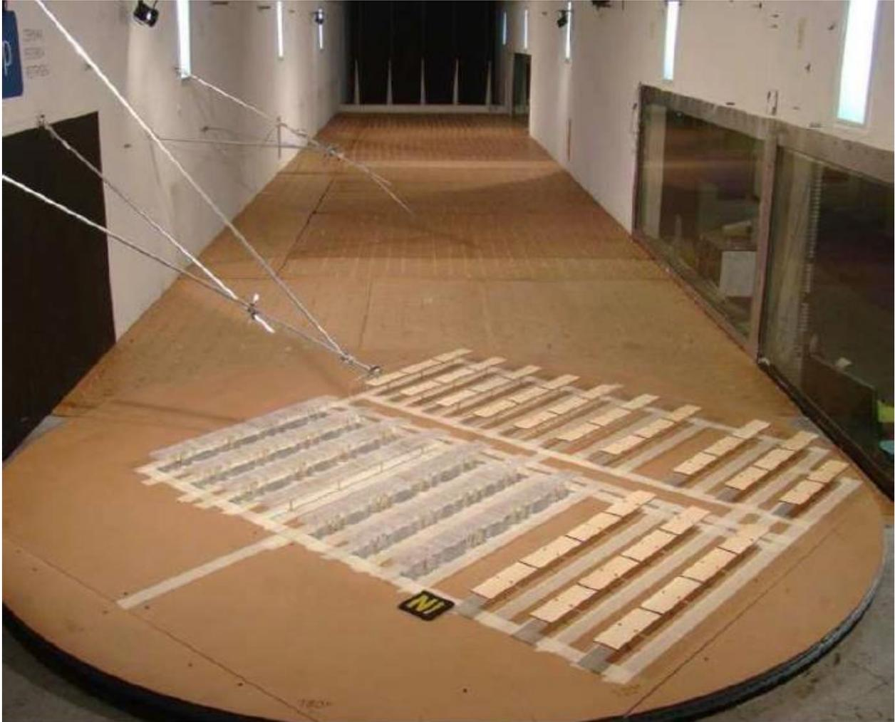
Figure 1: SCORPIUS Scaled model of typical solar arrays in boundary layer wind tunnel (©SCORPIUS)
