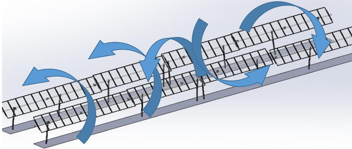
Figure 3: Schematic Representation of Uneven Twisting Torque on Line of Arrays
